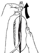
3. Pull cord halfway through unit. (Example: For 50 ft. cord, pull 25 ft. through.) Cordpro will then be in middle of cord.
