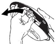
2. Flex open opposite side wall and pull cord end all the way through and out of the opening.
