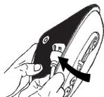
1. At eyelet tab, flex open one side wall and insert cord end through hole in divider.
